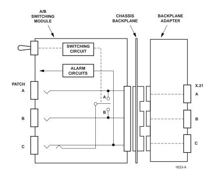
Figure 4-6. A/B Switching Block Diagram
